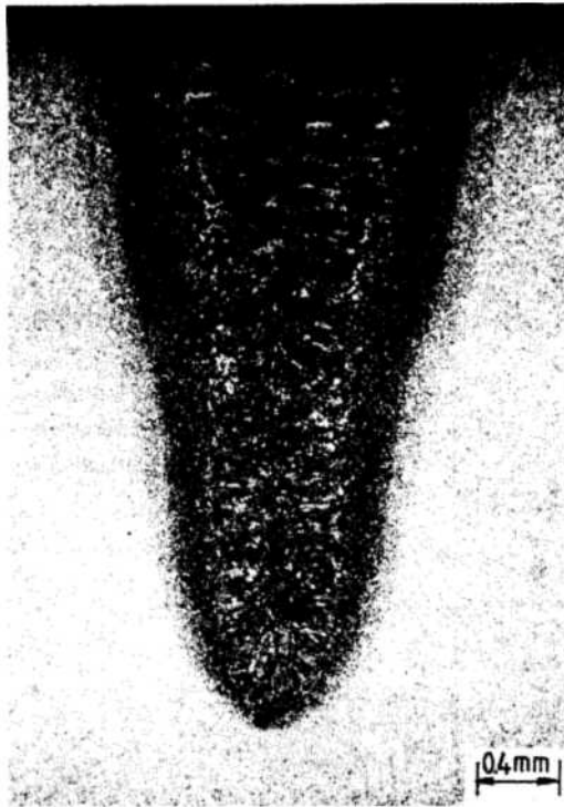
(a) P=2.0\text{kW} , v=1.5\text{m/min} , carbon steel
