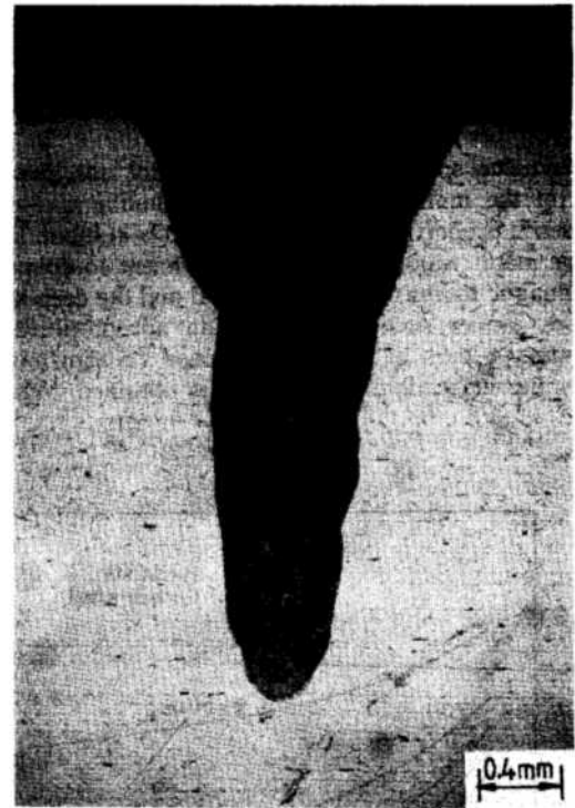
(b) P=2.0\text{kW} , v=1.5\text{m/min} , AISI 316 steel
